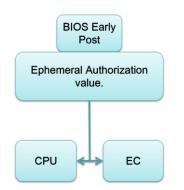
BIOS has to generate and store the ephemeral authentication value in the CPU and the EC . BIOS has to erase all records of this value outside of the CPU and the EC.
